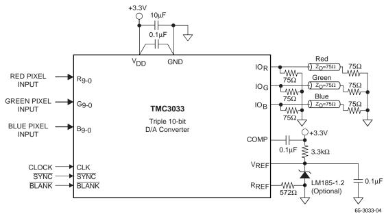
Figure 4. Typical Interface Circuit
