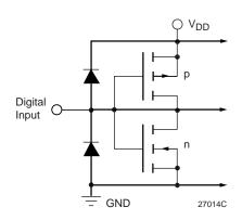
Figure 2. Equivalent Digital Input Circuit
