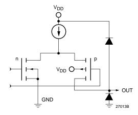
Figure 3. Equivalent Analog Output Circuit
