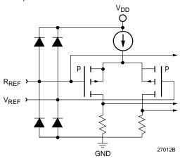
Figure 4. Equivalent Analog Input Circuit
